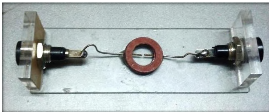
Fig. 2. Electrode chamber of dielectrophoresis
